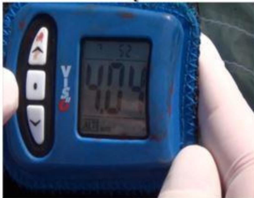
Fig. 7 The altimeter. The display of the different functions/data is selected with the scroll keys keys, on the device used for our example these are located on the left of the display.
