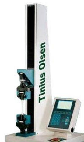
Figure 1: H5KT dynamometer
