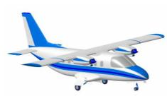
AeroTAXI is a project for a 12 pax subcommuter scale twin engine aircraft (CS-23) as main vector for a next generation of air transportation system at regional scale. This project, founded by national R&D program, is a cooperation with Romanian major establishments INAv, AVIOANE Craiova and University Politehnica Bucharest and is now in the phase of delivering a specimen for fatigue test.
