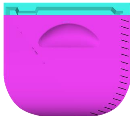
Figure 3 : Vortex generators (VG’s) on A320 MLG door. Courtesy of FOI.
